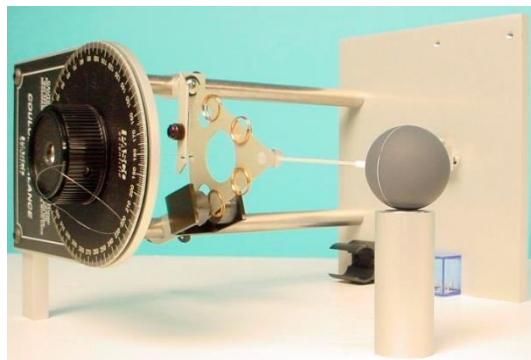
Figure 6. Calibrating the Torsion Balance
