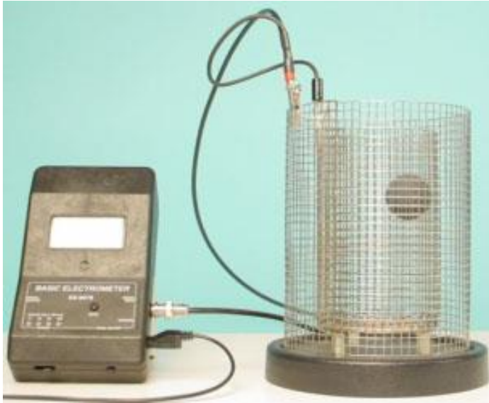
Figure 8. Measuring the Charge with an Electrometer and a Faraday Ice Pail
