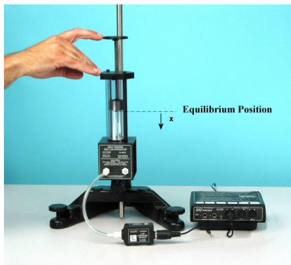
Figure 1: The piston is plucked by hand.
